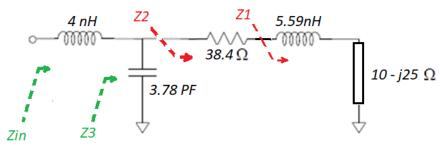
3. Compute the normalized impedance/admittance points (ZL,Z1,Z2,Z3 and Zin) in figure below; locate these points on impedance/admittance Smith chart and show the solution track on smith. find Zin,  $\Gamma$ in, VSWR. f=159MHz
